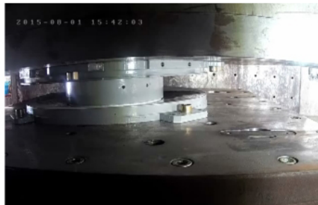
Dynamic tests for the Sliding Pendulum Isolators for the Bursa Hospital, Turkey, executed in our laboratory
