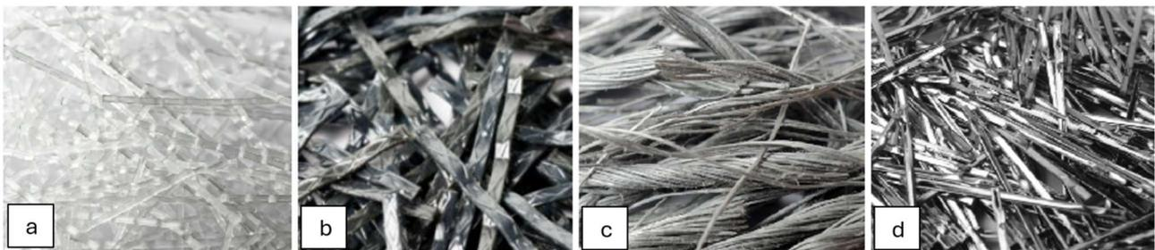
**Figura 4** – Fibre tipo: (a) FIBERCOLL FLEX 40, (b) FIBERCOLL FLAT, (c) FIBERCOLL TOP, (c) FIBERCOLL STEEL 60/65
