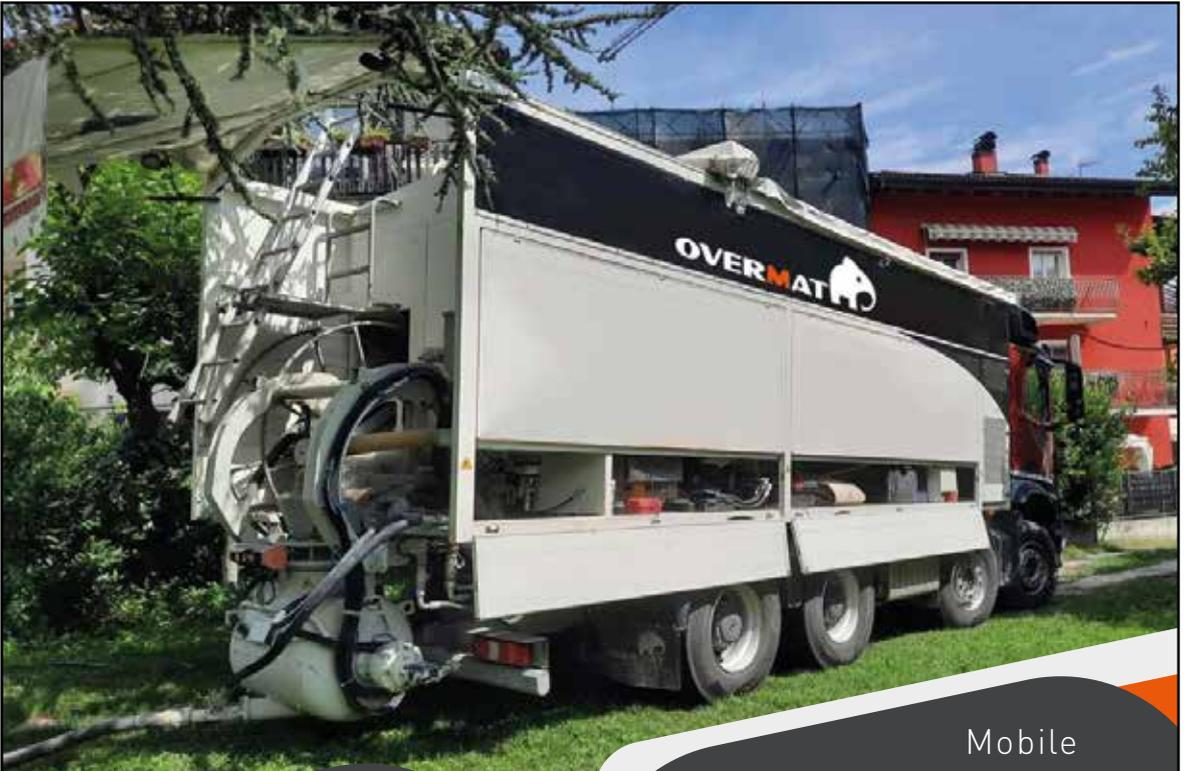
Mobile units for mixing and pumping screed, liquid self-levelling, foam and EPS concrete directly on the job site
