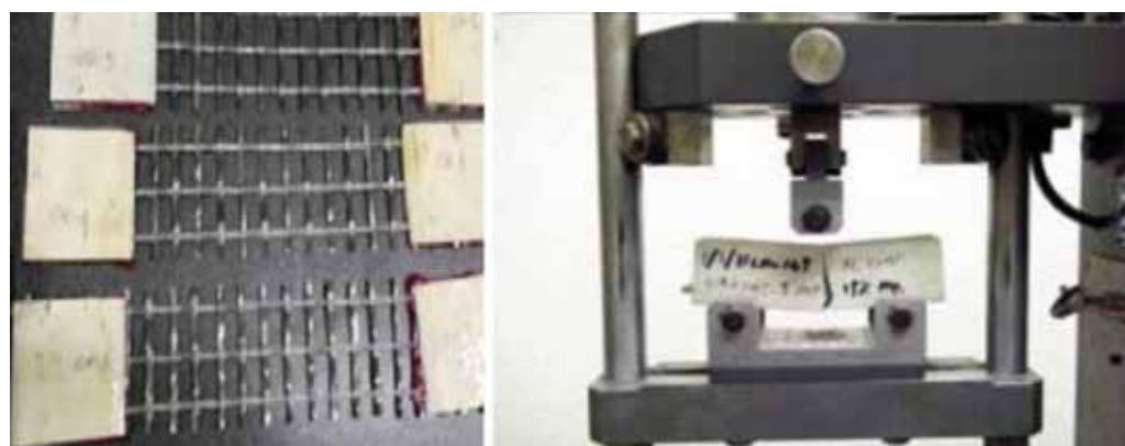
Figure 1 – Characterization of the reinforcement components: a) strips of GFRP grid and b) bending test of a mortar specimen
