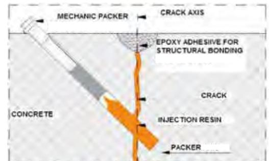
Fig. 2. Cracks' sealing procedure
