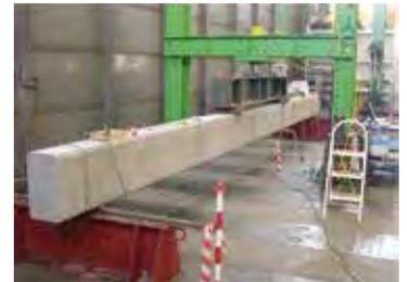
Fig. 2. Typical beam before execution of test
