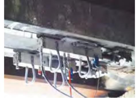
Fig. 8. Hydraulic jack pushing the mobile steel anchorage contrasting with the steel bolted plate.
